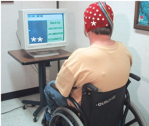
FIGURE 4. Example of an EEG-based BCI platform. Notable elements include the electrode cap worn (asterisk) by the subject and the viewer screen (double asterisks) for which the subject controls the cursor on the screen (BCI computer not shown) by various EEG signals and signal processing methods (i.e., sensorimotor rhythms, SCP, or P300 paradigm) (89).
