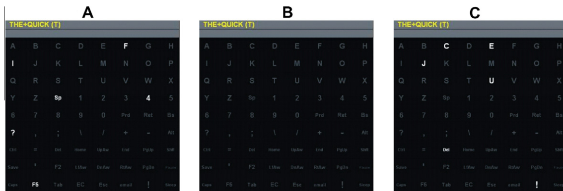
Fig. 1. The P300 Speller matrix. A. A group of six characters flashes. This is the on-period. B. No characters are highlighted. This is the off-period. One divided by the combined duration of the on- and offline periods in seconds is the flash rate. C. A new group of six characters flashes.
