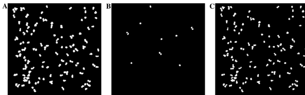
Fig. 7. (A) Same as Fig. 6C, (B) result of erosion-dilation, (C) result of region growing/watershed on a distance map for segmentation of clusters.
